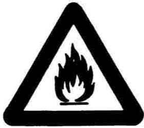
Flammable material or high temperature (1)
